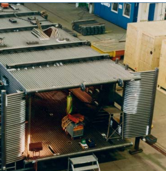
Boiler for a municipal-waste incinerator. The company is focusing on components for energy and power-plant engineering, and process-related plant engineering.
